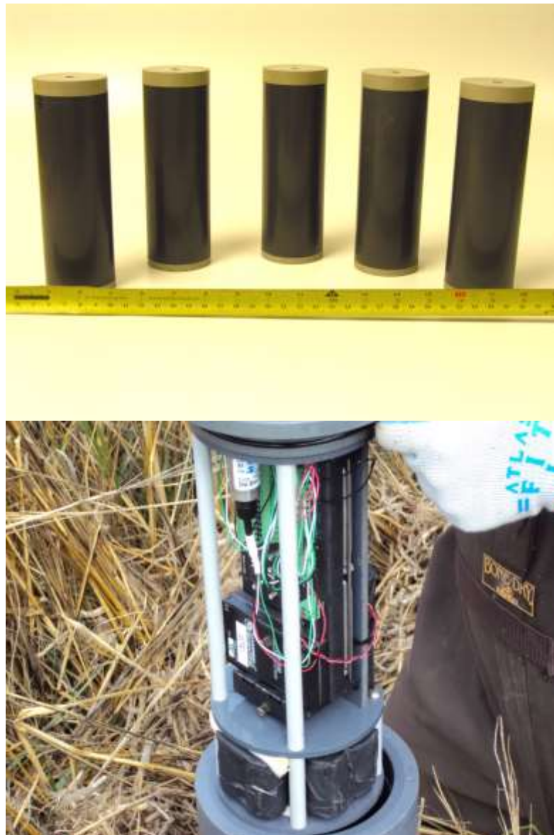
Fig. 4.12. (top) Marsh gages housing with pressure transducer inside, and (bottom) Inside of the data logger assembly with integrated pressure transducer.
