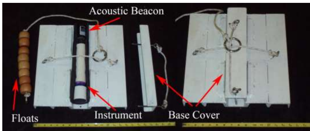
Fig. 4.10. Gage used to measure hurricane waves.
