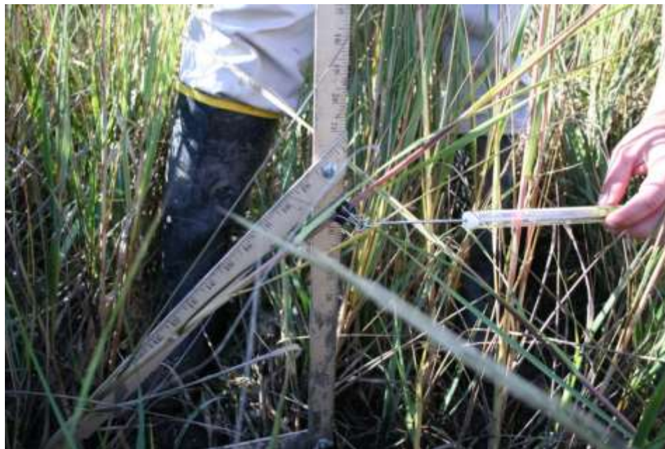
Fig. 5.3. Measuring plant bending force.
