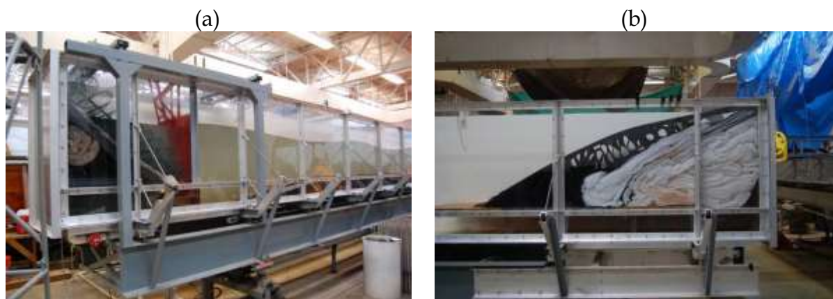
Fig. 3.7. (a) The wave generator and (b) wave absorber.
