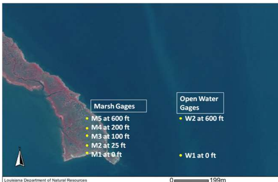
Fig. 4.26. Arrays of marsh and open water gages in Terrebonne Bay during Jul-Dec, 2010 (North-South alignment).
