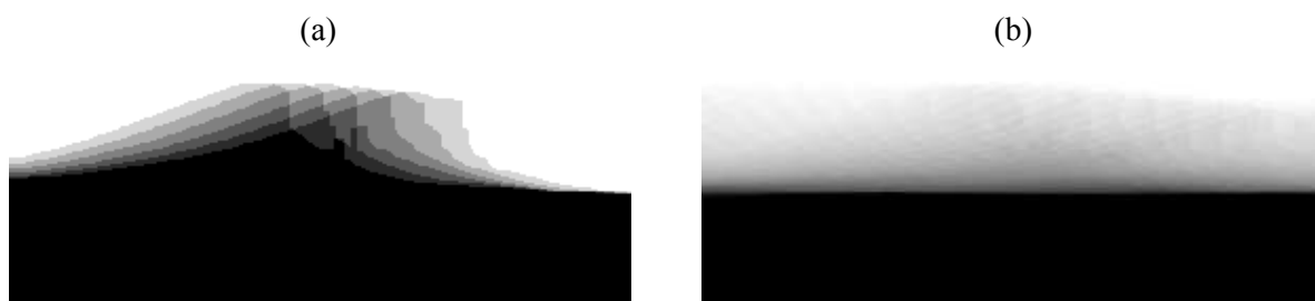
Fig. 3.27. A portion of the average (a) 5 frames and (b) 48 frames for breaking waves over the sloping beach ( T = 1.6 s, H = 0.14 m and h = 0.4 m).
