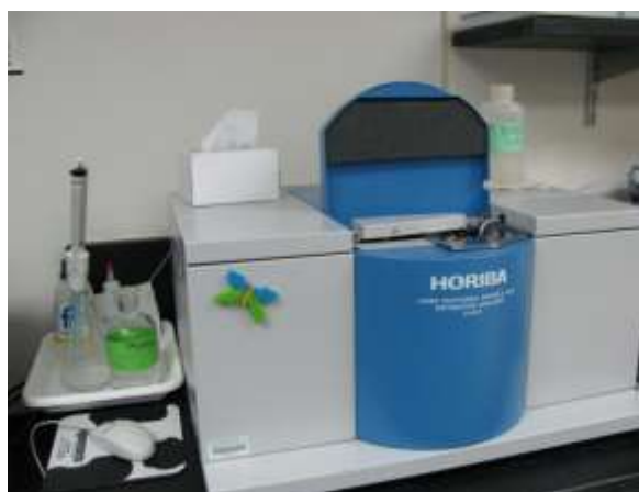
Fig. 5.26. Horriba LA-910 Particle Size Analyzer (USDA-ARS National Sedimentation Lab).
