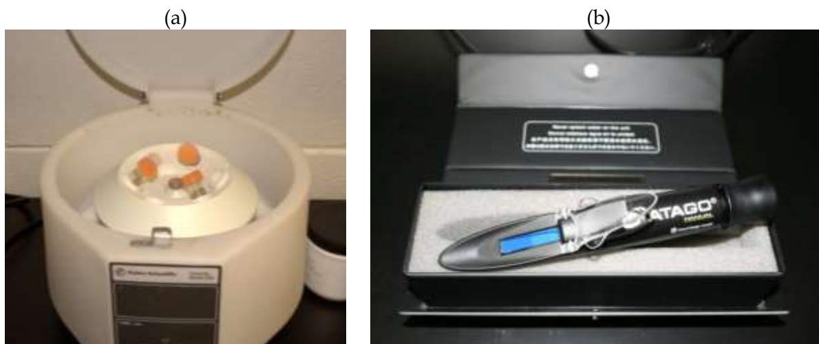
Fig. 5.6. (a) Centrifuge used to separate soil solids from pore water and (b) handheld salinity refractometer.
