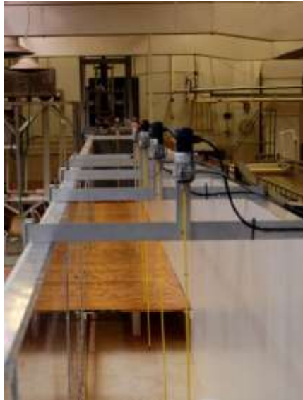
Fig. 3.20. Level sensors mounted on wave tank.
