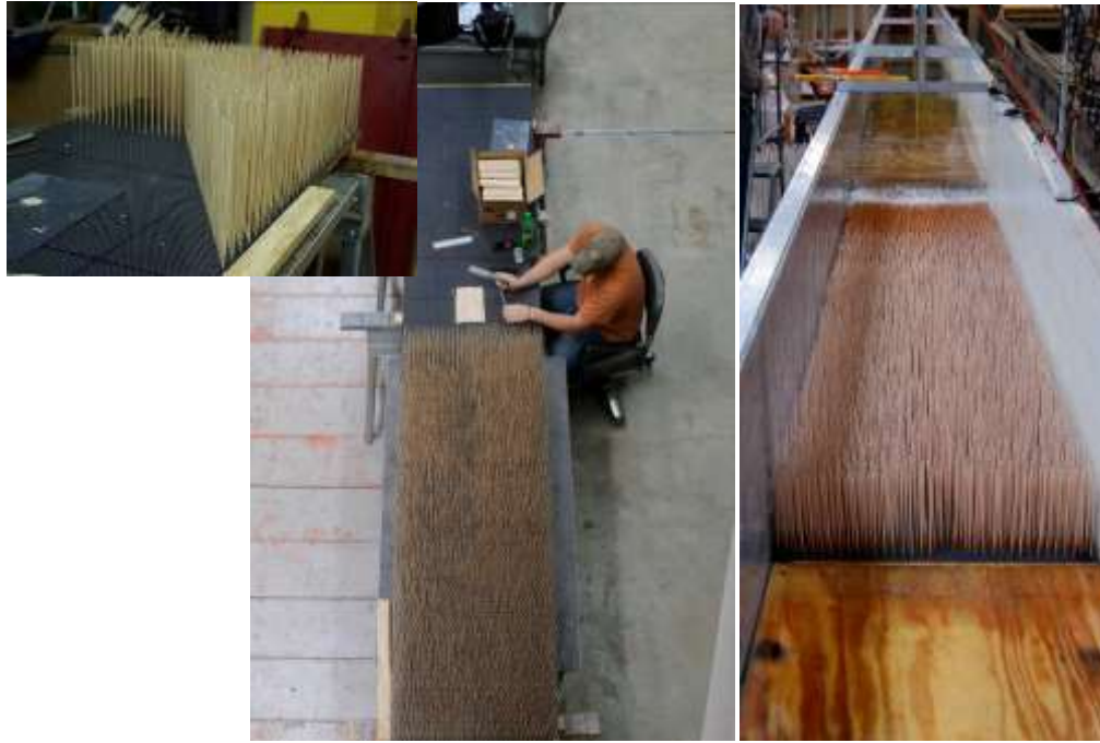
Fig. 3.13. Construction of the rigid vegetation elements
