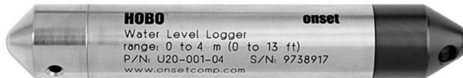
Fig. 4.9. Photo of gage used to measure hurricane surge.
